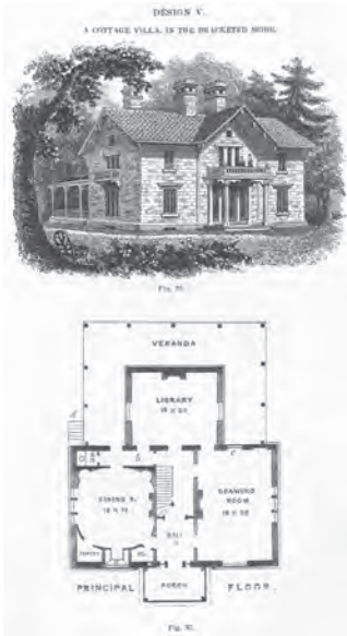
Cottage Villa, in the Bracketed Mode by Downing – Cottage Residences, 1842, Design V – View and Floor Plan
